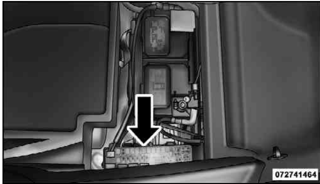
Rear Power Distribution Center
