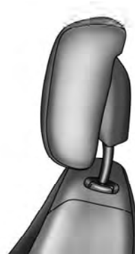
Active Head Restraint (Normal Position)
