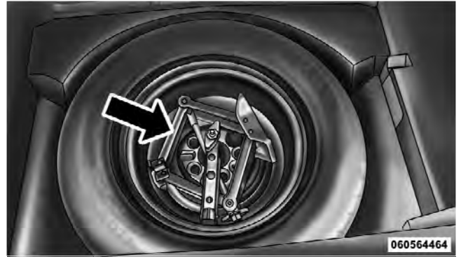
Spare Tire And Jack Stowage Without Tie Down Strap Spare Tire Stowage
