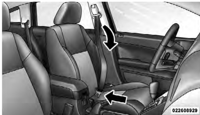
Inserting Latch Plate Into Buckle
