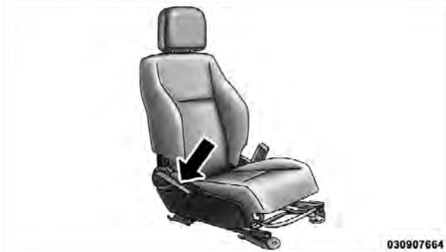
Fold-Flat Front Passenger Seat Lever
