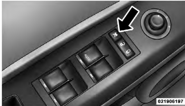
Window Lockout Switch
