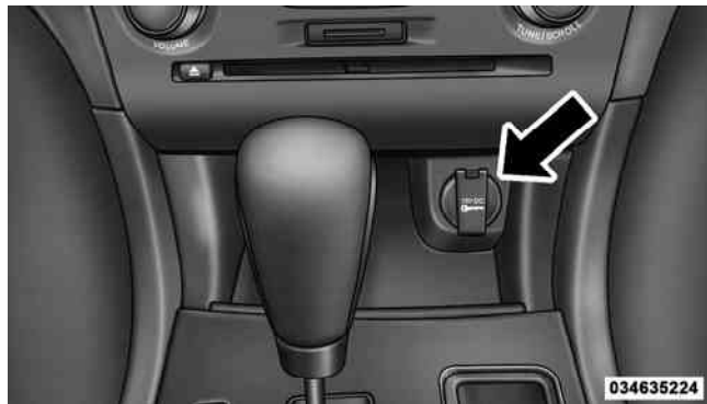
Front Power Outlet
