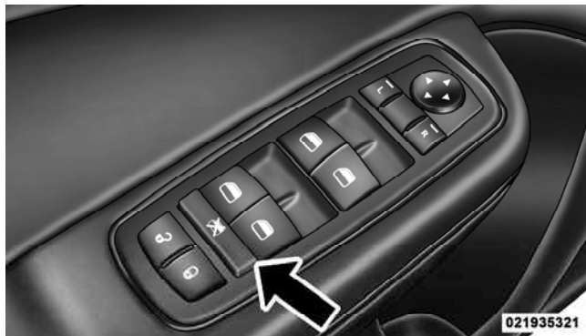
Window Lockout Switch
