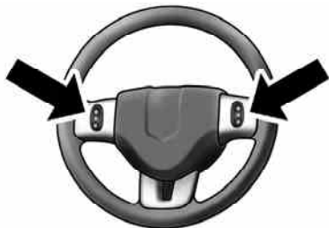
Remote Sound System Controls
