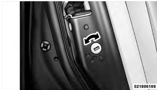
Child-Protection Door Lock Function
