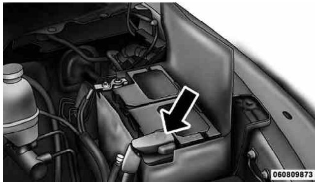
Positive Battery Post
