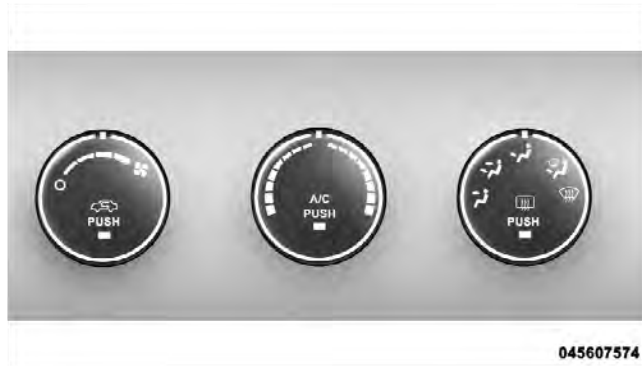
Manual Temperature Control
