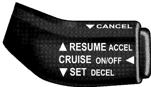
Electronic Speed Control Lever
