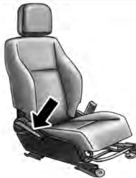
Fold-Flat Front Passenger Seat Handle
