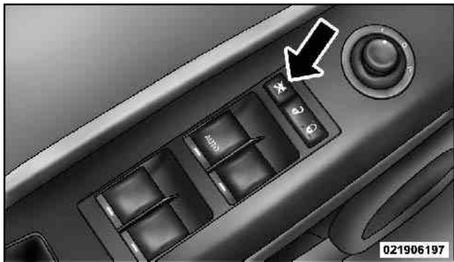
Window Lockout Switch
