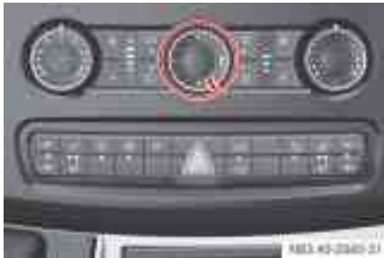
Air distribution control
