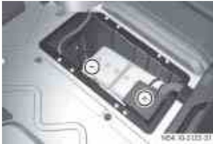
Starter battery in the driver's footwell
