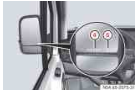
Warning display in the left-hand exterior mirror for the area to the rear left-hand side
