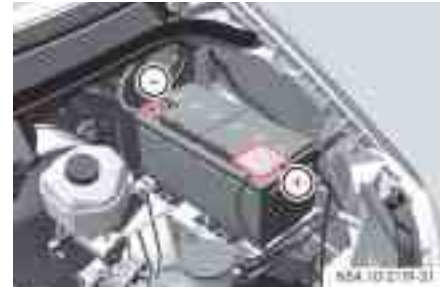
Auxiliary battery in the engine compartment
