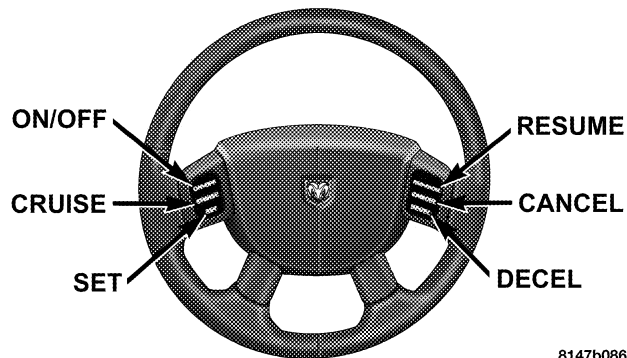
Speed Control Switches
