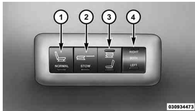
Rear Panel Power Switch Bank
