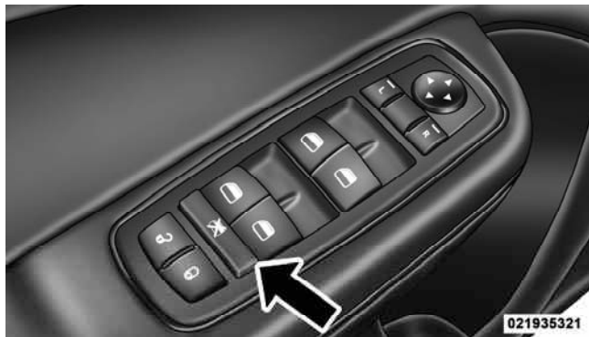
Window Lockout Switch
