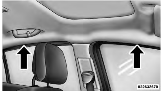
Side Airbag Inflatable Curtains (SABIC) Location
