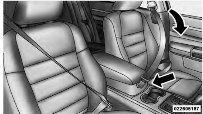
Removing Slack from Belt
