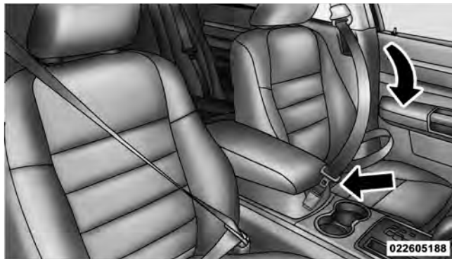
Inserting Latch Plate into Buckle
