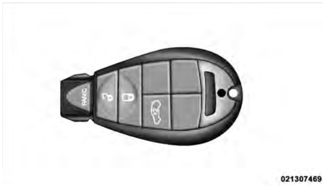
Key Fob with RKE Transmitter
