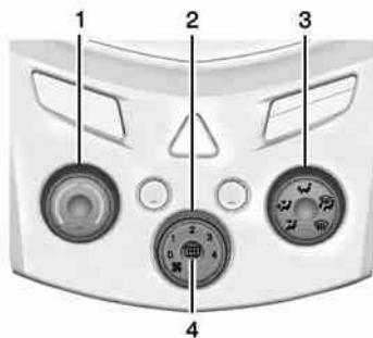
Climate Control System with Heater Only
