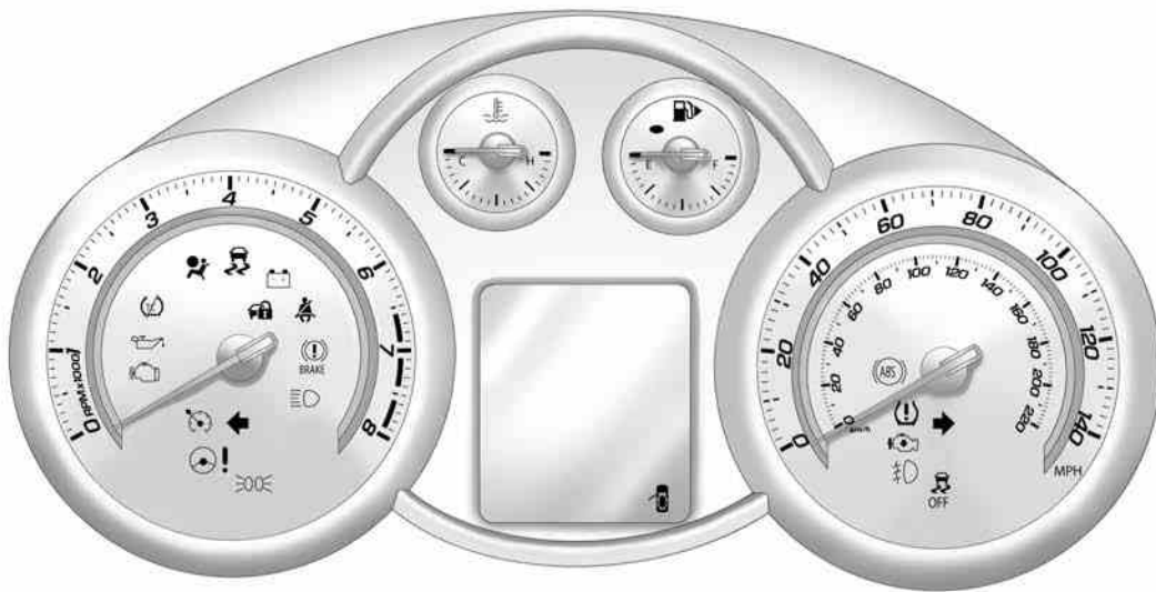
English Gas Cluster with Automatic Transmission Shown, Metric and Manual Transmission Similar
