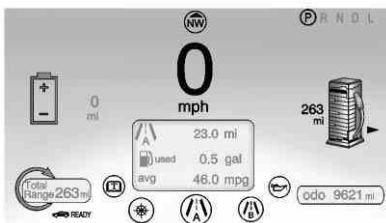
Simple Configuration in Extended Range Mode
