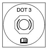
Your vehicle has one reservoir for both the brake and clutch hydraulic systems. It is filled with DOT-3 brake fluid. See Engine Compartment Overview on page 5-12 for the location of the reservoir.
