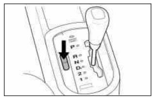
Press the HOLD button on the shift lever console to turn on hold mode. Press the button again to turn off hold mode, and return to normal automatic transaxle operation. While on, the HOLD light on the secondary information center will light up. See *Hold Mode Light on page 3-34*.
