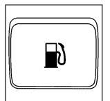
To open the fuel filler door, pull up on the release lever with this symbol on it. It is located on the floor on the outboard side of the driver's seat.
