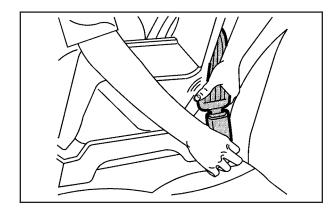
3. Buckle the belt. Be sure the latch plate clicks when you put it into the buckle. This means you are using the correct buckle. Also, make sure the release button is positioned so you would be able to unbuckle the safety belt quickly if you ever had to.
