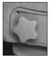
If your vehicle has a lumbar adjustment, the knob is located on the outboard side of the seat cushion.
