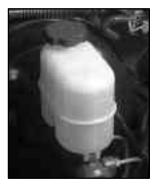
Your brake master cylinder reservoir is located in the rear of the engine compartment on the driver's side of the vehicle.
