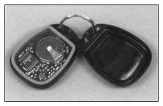
1. Insert a dime, or similar object, in the slot between the covers of the transmitter housing near the key ring hole. Remove the bottom by twisting the dime.
