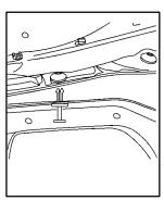
3. Pull the push-pins and lower air dam assembly away from the retainers until the lower air dam is free.
