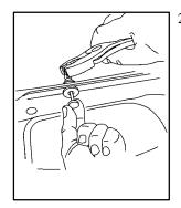
2. While continuing to pull downward on the push-pin, squeeze and turn the expandable end of the push-pin with a tool until it releases from the retainer.
