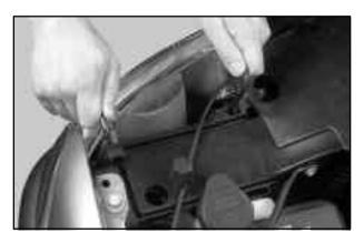
1. Remove the two pins on the top of the headlamp assembly. To remove the pins, turn the outer pin outward and pull it straight up. To remove the inner pin, turn it in and pull it straight up.
