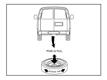
6. Make sure the tire is stored securely. Push, pull, and then try to rotate or turn the tire. If the tire moves, use the wheel wrench to tighten the cable.
