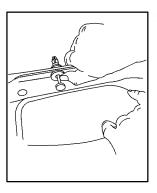
Line up each push-pin with its intended retainer and push the washer portion of the push-pin towards the retainer until it locks into place.
