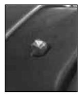
The hazard warning flasher is located at the top of the steering column.
