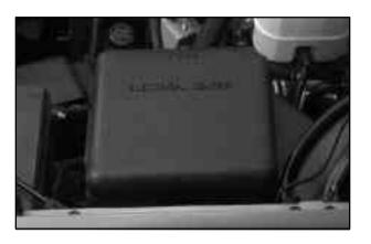
The underhood fuse block is located on the driver's side of the vehicle near the battery. Lift the cover for access to the fuse/relay block.
