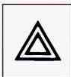
Hazard Warning Flasher
