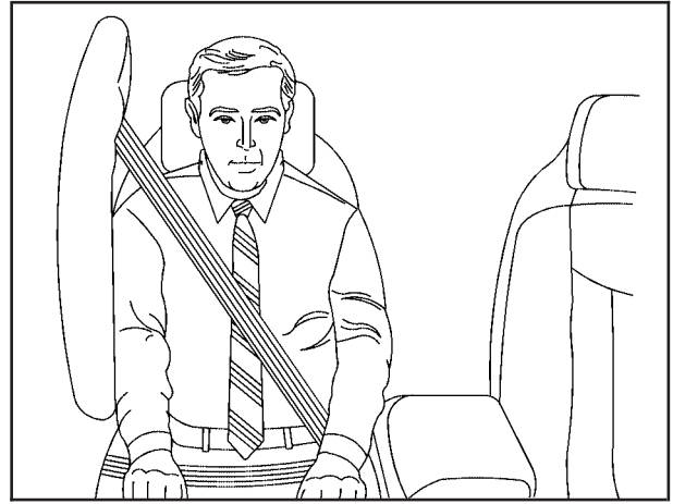
The passenger's side impact airbag is in the side of the passenger's seatback closest to the door.
