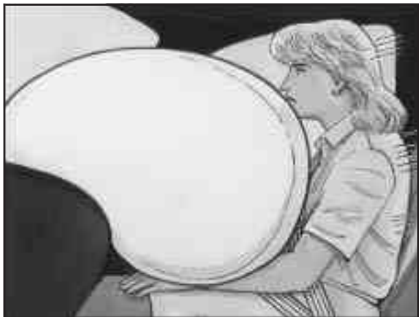
The right front passenger's frontal airbag is in the instrument panel on the passenger's side.
