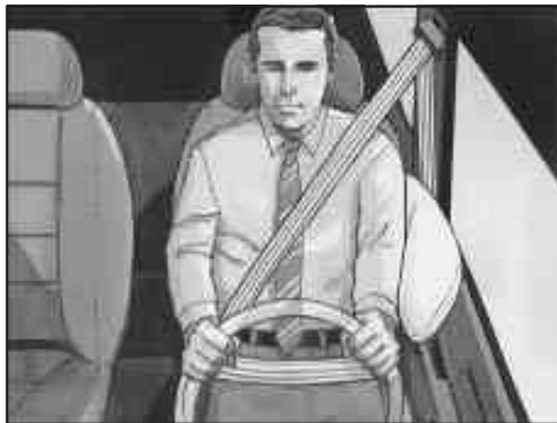
The seat-mounted side impact airbag for the driver is in the side of the driver's seatback closest to the door.
