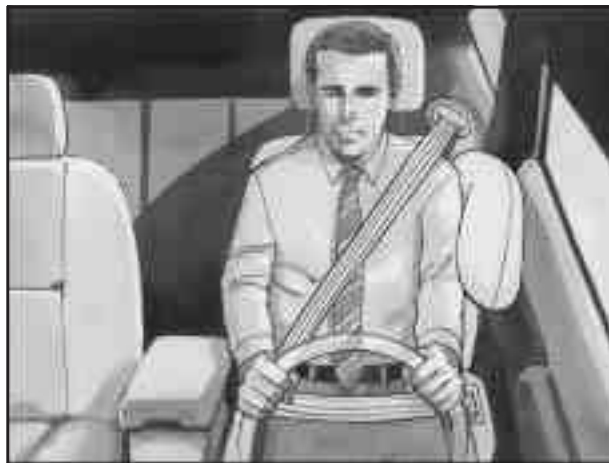
The driver's seat-mounted side impact airbag is in the side of the driver's seatback closest to the door.
