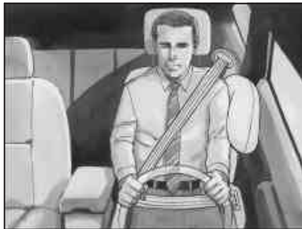
The driver's seat-mounted side impact air bag is in the side of the driver's seatback closest to the door.
