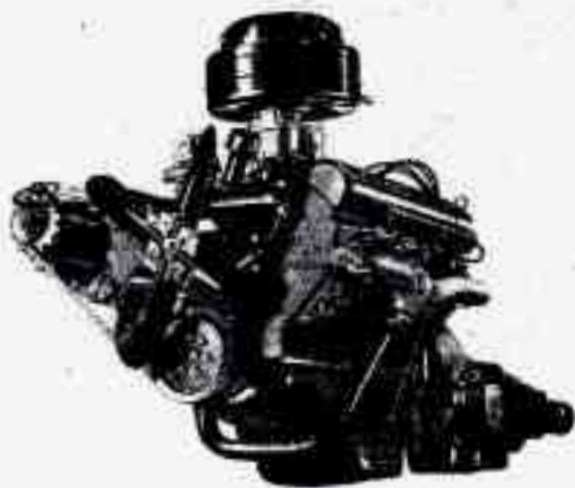
1949 Overhead Valve High Compression V8 Engine
